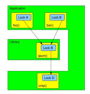
Figure 7.7: Layered Locking Hierarchy for qsort()
