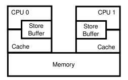
Figure 15.1: System Architecture With Store Buffers
