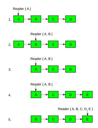
Figure 9.15: Multiple RCU Data-Structure Versions
