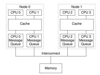
Figure C.8: Example Ordering-Hostile Architecture
