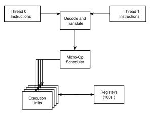
Figure 3.4: Rough View of Modern Micro-Architecture
