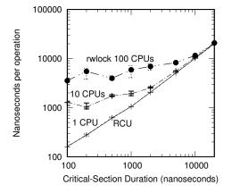
**Figure 9.27:** Comparison of RCU to Reader-Writer Locking as Function of Critical-Section Duration, 192 CPUs
