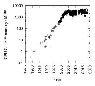
Figure 2.1: MIPS/Clock-Frequency Trend for Intel CPUs
