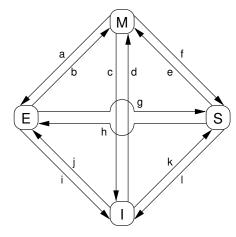
Figure C.3: MESI Cache-Coherency State Diagram
