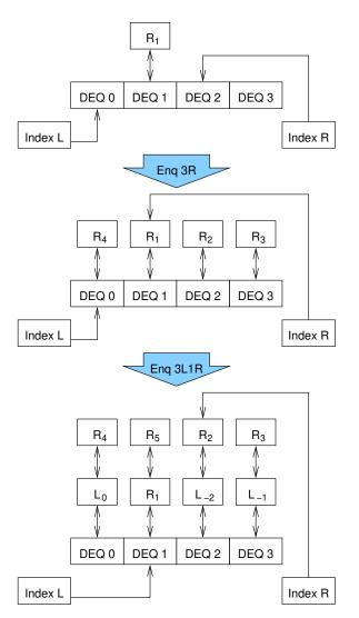
Figure 6.8: Hashed Double-Ended Queue After Insertions
