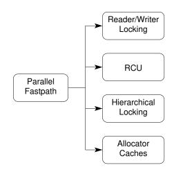
Figure 6.18: Parallel-Fastpath Design Patterns
