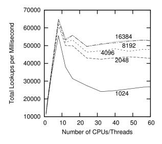
Figure 10.9: Read-Only Hash-Table Performance For Schrödinger's Zoo, Varying Buckets
