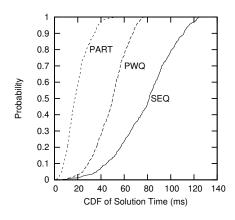
Figure 6.39: CDF of Solution Times For SEQ, PWQ, and PART
