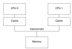
Figure 14.1: Modern Computer System Cache Structure
