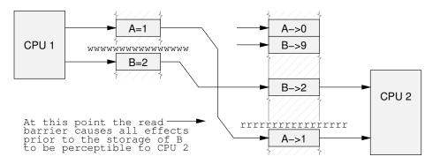
Figure 14.11: Read Barrier Supplied
