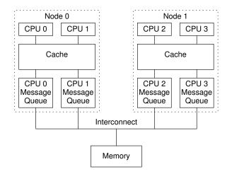
Figure C.8: Example Ordering-Hostile Architecture
