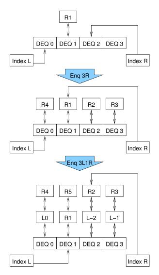
Figure 6.8: Hashed Double-Ended Queue After Insertions
