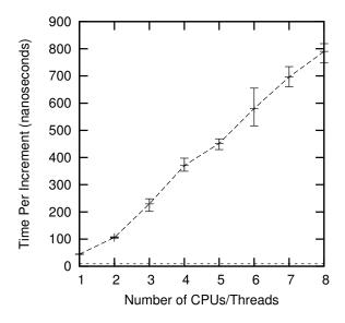
Figure 5.3: Atomic Increment Scalability on Nehalem
