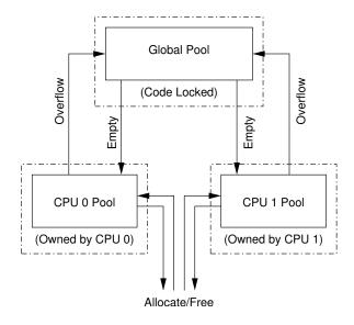
Figure 6.27: Allocator Cache Schematic
