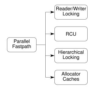
Figure 6.24: Parallel-Fastpath Design Patterns
