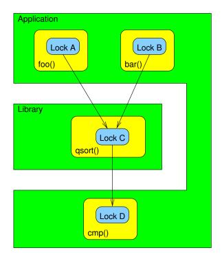
Figure 7.6: Layered Locking Hierarchy for qsort()
