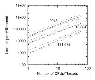
Figure 10.29: Overhead of Resizing Hash Tables
