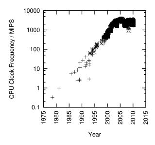
Figure 2.1: MIPS/Clock-Frequency Trend for Intel CPUs
