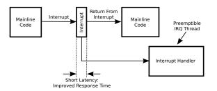
Figure 15.13: Threaded Interrupt Handler
