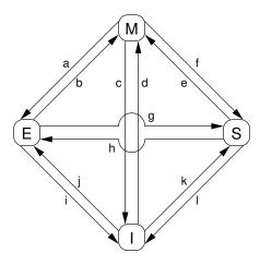
Figure C.3: MESI Cache-Coherency State Diagram
