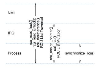
Figure 9.35: RCU API Usage Constraints
