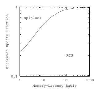
Figure 17.6: Breakevens vs. r,  $\lambda$  Large, Four CPUs
