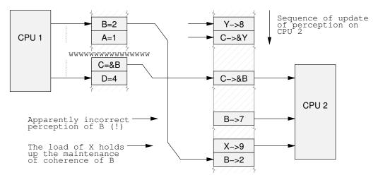
Figure 14.8: Data Dependency Barrier Omitted
