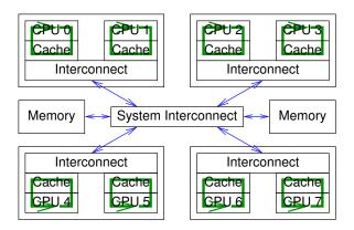
Figure 4.7: Data Flow For Per-Thread Increment
