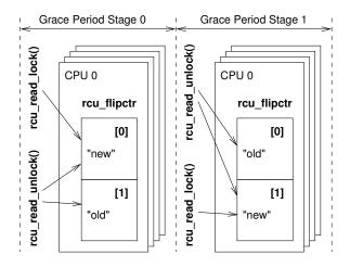
Figure D.61: Preemptible RCU Counter Flip Operation
