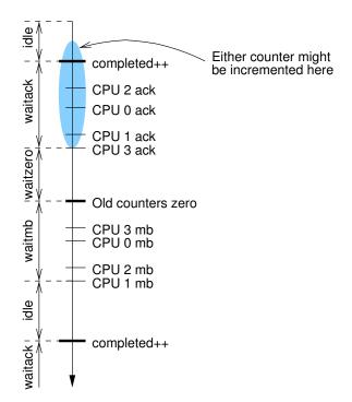
Figure D.64: Preemptible RCU State Machine Timeline
