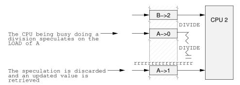
Figure 13.16: Speculative Load Cancelled by Barrier
