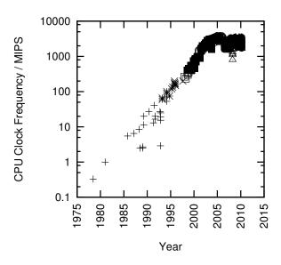
Figure 1.1: MIPS/Clock-Frequency Trend for Intel CPUs
