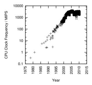
Figure 5.14: MIPS/Clock-Frequency Trend for Intel CPUs
