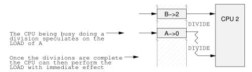
Figure 13.14: Speculative Load
