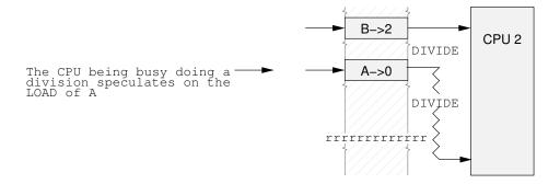
Figure 13.15: Speculative Load and Barrier
