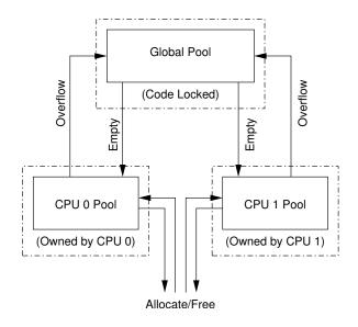
Figure 5.27: Allocator Cache Schematic
