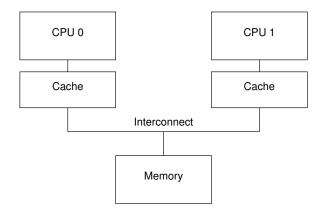
Figure 13.1: Modern Computer System Cache Structure
