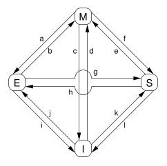
Figure C.3: MESI Cache-Coherency State Diagram
