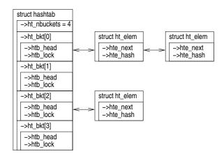
Figure 9.2: Hash-Table Data-Structure Diagram
