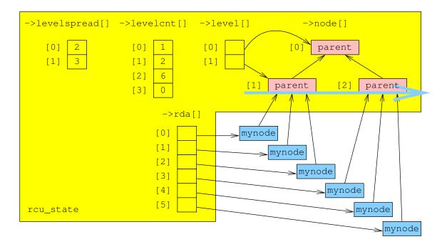
Figure D.52: Scanning Leaf rcu\_node Structures
