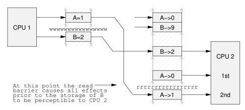
Figure 13.12: Read Barrier Supplied, Double Load
