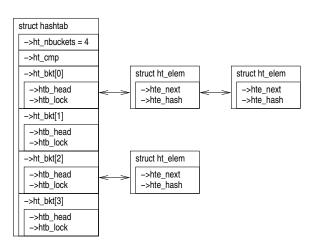
Figure 10.1: Hash-Table Data-Structure Diagram
