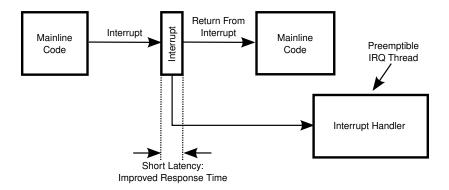
Figure 14.13: Threaded Interrupt Handler
