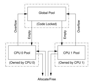
Figure 6.19: Allocator Cache Schematic
