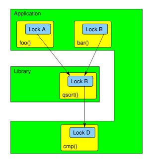
Figure 7.7: Layered Locking Hierarchy for qsort()
