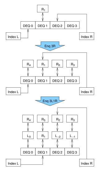
Figure 6.8: Hashed Double-Ended Queue After Insertions
