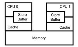
Figure 15.1: System Architecture With Store Buffers
