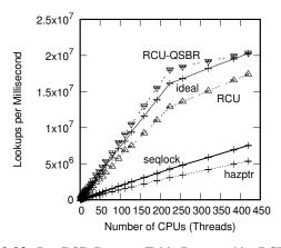
Figure 9.22: Pre-BSD Routing Table Protected by RCU QSBR
