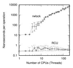
Figure 9.25: Performance Advantage of RCU Over Reader-Writer Locking
