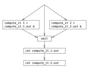
Figure 4.1: Execution Diagram for Parallel Shell Execution
