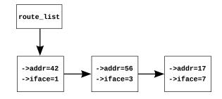
Figure 9.1: Pre-BSD Packet Routing List
