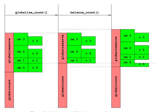
Figure 5.6: Schematic of Globalization and Balancing
