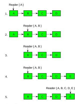
Figure 9.15: Multiple RCU Data-Structure Versions
