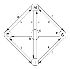
Figure C.3: MESI Cache-Coherency State Diagram
