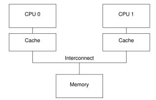
Figure C.1: Modern Computer System Cache Structure
