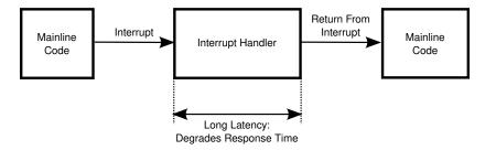
Figure 14.12: Non-Threaded Interrupt Handler
