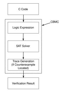
Figure 12.2: CBMC Processing Flow
