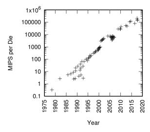
Figure 2.2: MIPS per Die for Intel CPUs
