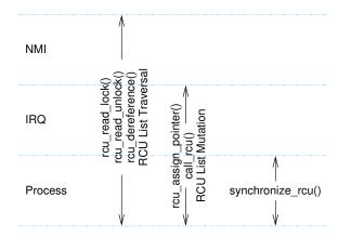
Figure 9.20: RCU API Usage Constraints
