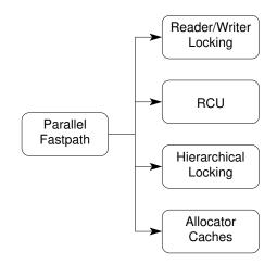
Figure 6.18: Parallel-Fastpath Design Patterns
