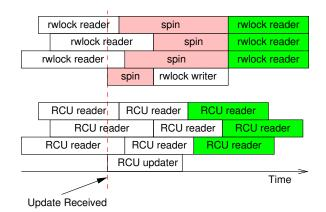
Figure 9.28: Response Time of RCU vs. Reader-Writer Locking
