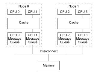
Figure C.8: Example Ordering-Hostile Architecture
