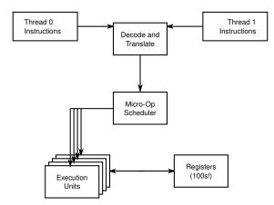
Figure 3.4: Rough View of Modern Micro-Architecture
