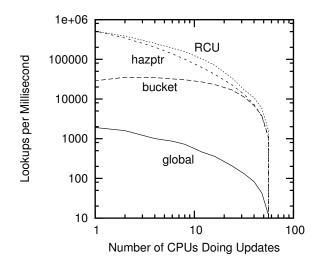
Figure 9.16: Read-Side RCU-Protected Hash-Table Performance For Schrödinger's Zoo at 60 CPUs
