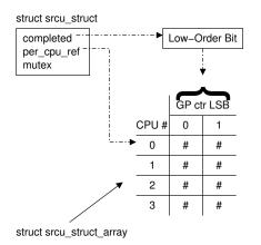
Figure D.5: SRCU Data-Structure Diagram
