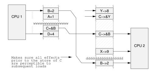
Figure 13.9: Data Dependency Barrier Supplied
