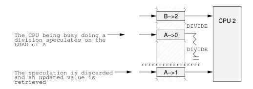
Figure 13.16: Speculative Load Cancelled by Barrier
