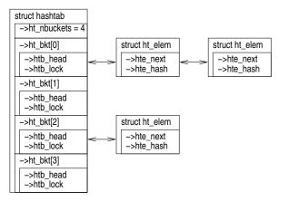
Figure 9.2: Hash-Table Data-Structure Diagram
