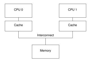
Figure C.1: Modern Computer System Cache Structure
