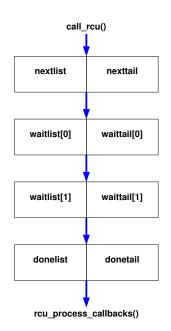
Figure D.62: Preemptible RCU Callback Flow
