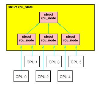
Figure D.12: Hierarchical RCU State
