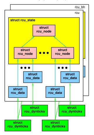
Figure D.17: Hierarchical RCU State With Dynticks
