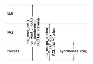
Figure 8.35: RCU API Usage Constraints
