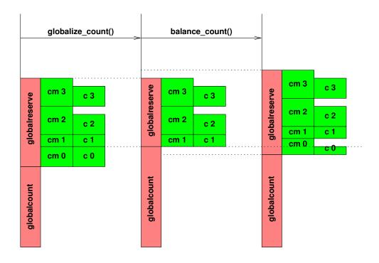
Figure 4.14: Schematic of Globalization and Balancing
