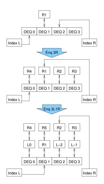
Figure 5.8: Hashed Double-Ended Queue After Insertions
