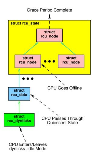
Figure D.19: RCU State Machine and Hierarchical RCU Data Structures
