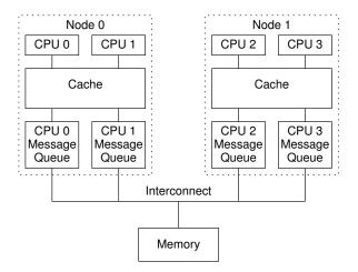
Figure C.8: Example Ordering-Hostile Architecture
