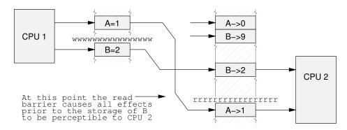
then the partial ordering imposed by CPU 1's write barrier will be perceived correctly by CPU 2, as shown in Figure 13.11.
