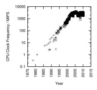
Figure 1.1: MIPS/Clock-Frequency Trend for Intel CPUs
