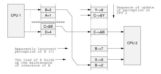
Figure 13.8: Data Dependency Barrier Omitted
