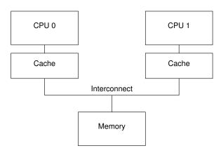
Figure 13.1: Modern Computer System Cache Structure
