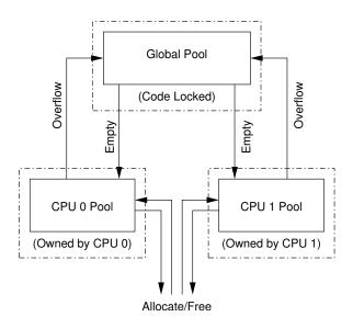
Figure 5.27: Allocator Cache Schematic
