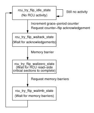
Figure D.63: Preemptible RCU State Machine
