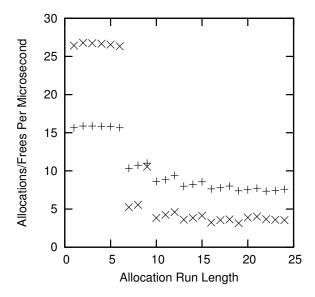
Figure 5.32: Allocator Cache Performance
