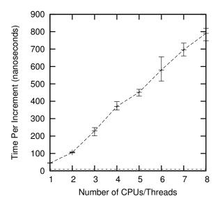
Figure 4.3: Atomic Increment Scalability on Nehalem
