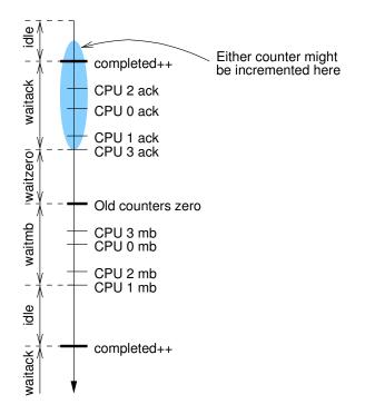
Figure D.64: Preemptible RCU State Machine Timeline
