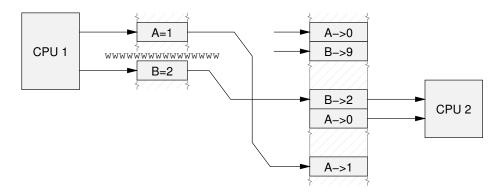
Figure 13.10: Read Barrier Needed
