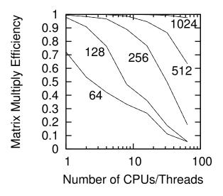
Figure 5.23: Matrix Multiply Efficiency
