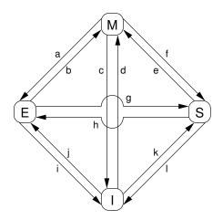
Figure C.3: MESI Cache-Coherency State Diagram
