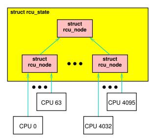
Figure D.15: Hierarchical RCU State 4,096 CPUs
