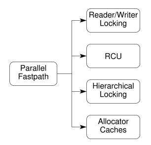
Figure 5.24: Parallel-Fastpath Design Patterns
