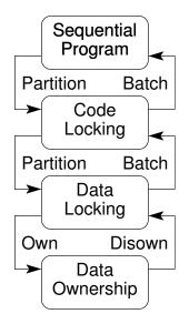
Figure 5.13: Design Patterns and Lock Granularity
