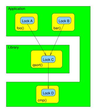
Figure 6.6: Layered Locking Hierarchy for qsort()
