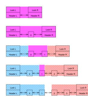
Figure 5.5: Double-Ended Queue With Left- and Right-Hand Locks
