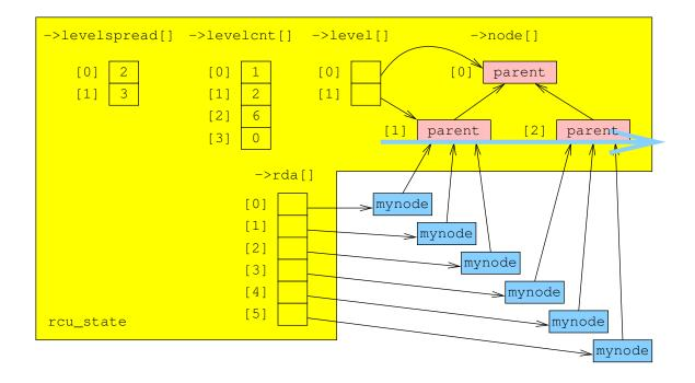
Figure D.52: Scanning Leaf rcu\_node Structures
