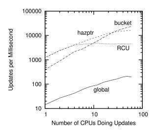
Figure 9.17: Update-Side RCU-Protected Hash-Table Performance For Schrödinger's Zoo at 60 CPUs
