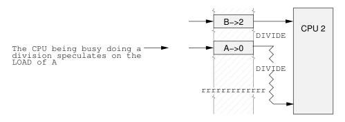
Figure 13.15: Speculative Load and Barrier
