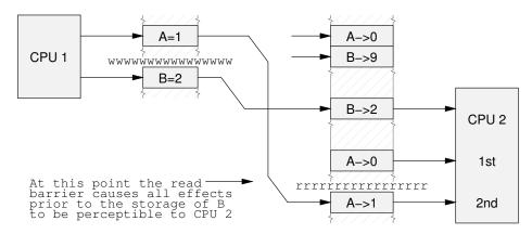
Figure 13.12: Read Barrier Supplied, Double Load
