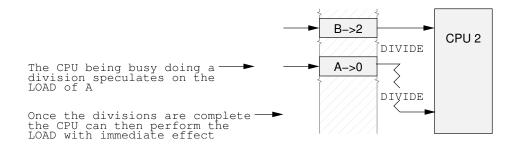
Figure 13.14: Speculative Load
