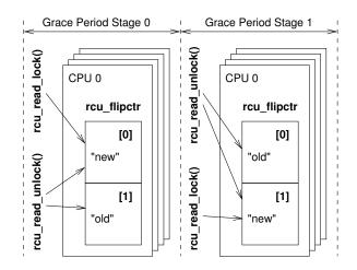
Figure D.61: Preemptible RCU Counter Flip Operation
