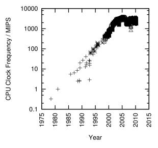
Figure 5.14: MIPS/Clock-Frequency Trend for Intel CPUs
