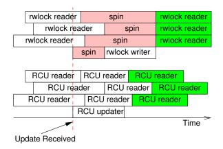
Figure 8.26: Response Time of RCU vs. Reader-Writer Locking
