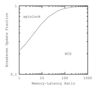
Figure 15.6: Breakevens vs. r,  $\lambda$  Large, Four CPUs
