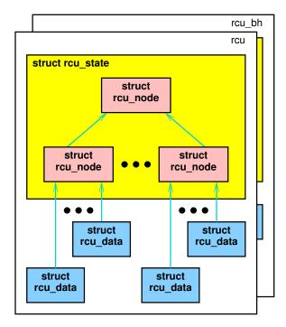
Figure D.16: Hierarchical RCU State With BH
