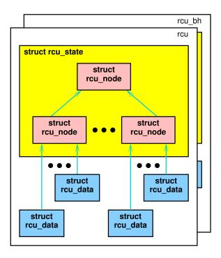
Figure D.16: Hierarchical RCU State With BH
