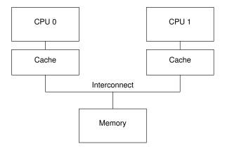
Figure C.1: Modern Computer System Cache Structure
