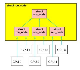
Figure D.12: Hierarchical RCU State
