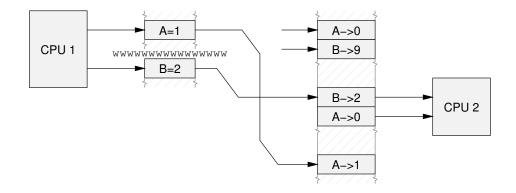
Figure 13.10: Read Barrier Needed
