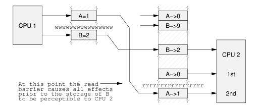
Figure 13.12: Read Barrier Supplied, Double Load
