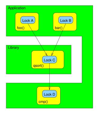
Figure 6.6: Layered Locking Hierarchy for qsort()
