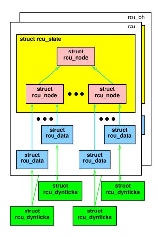
Figure D.17: Hierarchical RCU State With Dynticks
