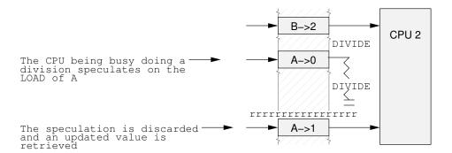
Figure 13.16: Speculative Load Cancelled by Barrier
