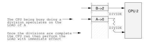
Figure 13.14: Speculative Load
