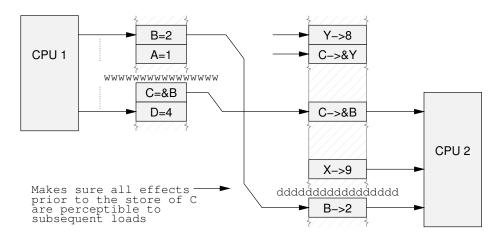
Figure 13.9: Data Dependency Barrier Supplied
