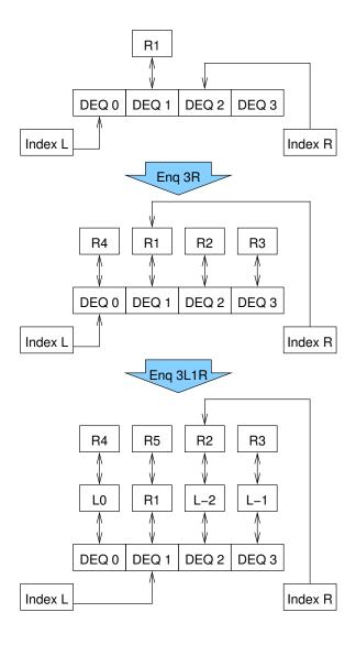
Figure 5.8: Hashed Double-Ended Queue After Insertions
