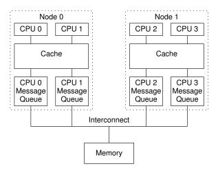
Figure C.8: Example Ordering-Hostile Architecture
