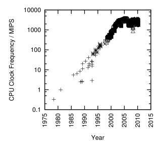
Figure 1.1: MIPS/Clock-Frequency Trend for Intel CPUs
