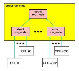
Figure D.15: Hierarchical RCU State 4,096 CPUs
