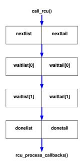
Figure D.62: Preemptible RCU Callback Flow
