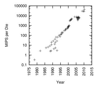
Figure 1.2: MIPS per Die for Intel CPUs
