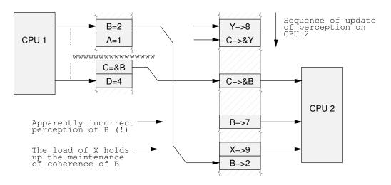
Figure 13.8: Data Dependency Barrier Omitted
