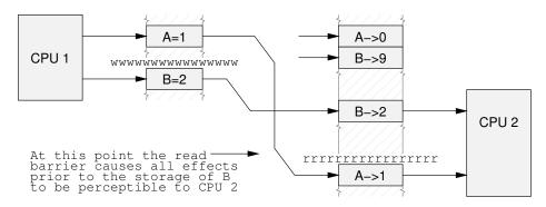
Figure 13.11: Read Barrier Supplied
