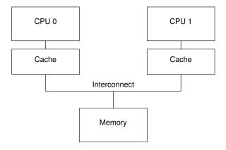
Figure 13.1: Modern Computer System Cache Structure
