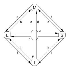
Figure C.3: MESI Cache-Coherency State Diagram
