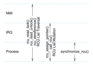
Figure 8.35: RCU API Usage Constraints
