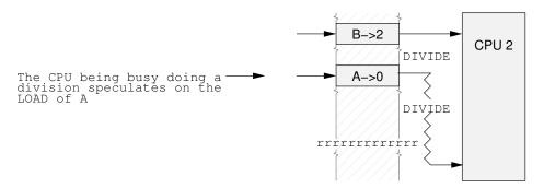
Figure 13.15: Speculative Load and Barrier
