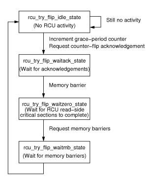
Figure D.63: Preemptible RCU State Machine
