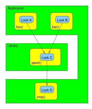
Figure 6.6: Layered Locking Hierarchy for qsort()
