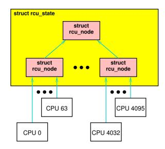
Figure D.15: Hierarchical RCU State 4,096 CPUs
