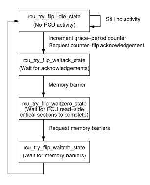
Figure D.63: Preemptible RCU State Machine
