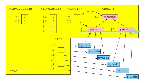
Figure D.52: Scanning Leaf rcu\_node Structures
