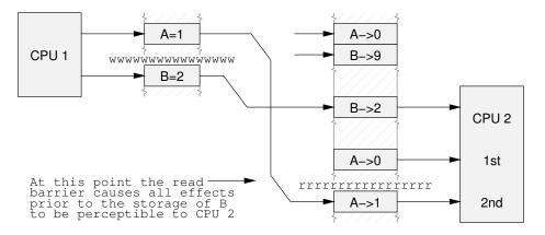
Figure 13.12: Read Barrier Supplied, Double Load
