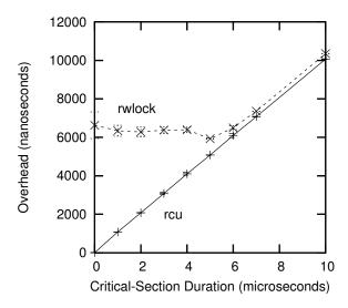
Figure 8.25: Comparison of RCU to Reader-Writer Locking as Function of Critical-Section Duration
