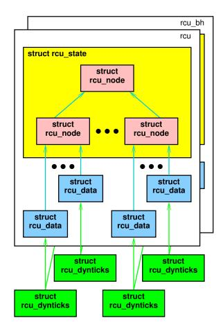
Figure D.17: Hierarchical RCU State With Dynticks
