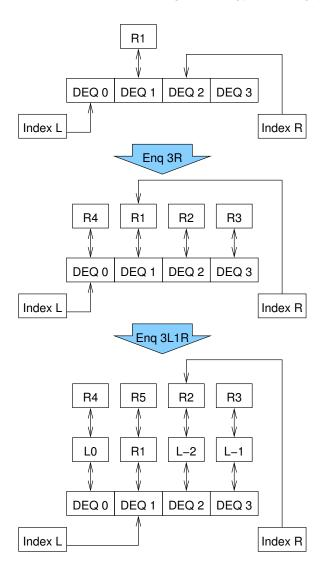
Figure 5.8: Hashed Double-Ended Queue After Insertions
