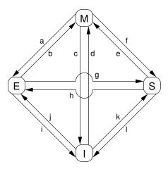
Figure C.3: MESI Cache-Coherency State Diagram
