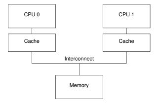
Figure 13.1: Modern Computer System Cache Structure
