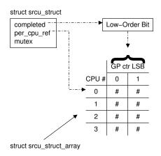
Figure D.5: SRCU Data-Structure Diagram
