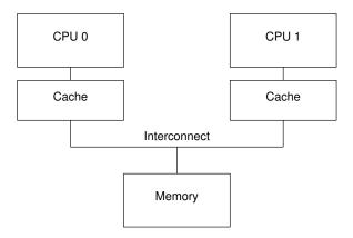
Figure C.1: Modern Computer System Cache Structure
