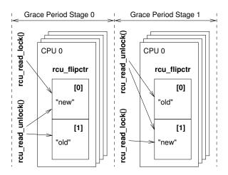
Figure D.61: Preemptible RCU Counter Flip Operation
