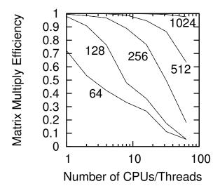
Figure 5.23: Matrix Multiply Efficiency
