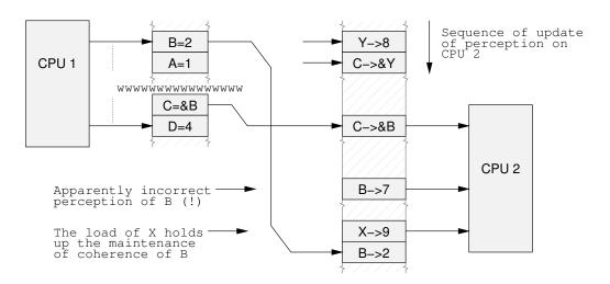
Figure 13.8: Data Dependency Barrier Omitted
