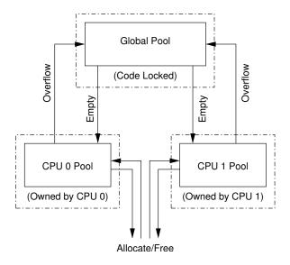
Figure 5.27: Allocator Cache Schematic
