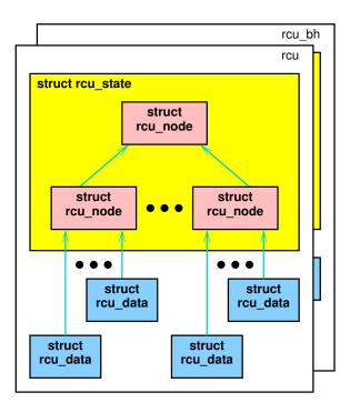
Figure D.16: Hierarchical RCU State With BH
