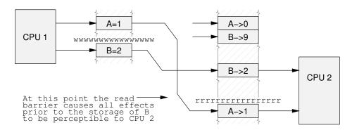
Figure 13.11: Read Barrier Supplied
