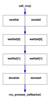
Figure D.62: Preemptible RCU Callback Flow
