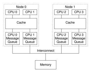
Figure C.8: Example Ordering-Hostile Architecture
