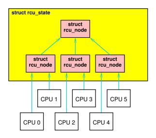
Figure D.12: Hierarchical RCU State
