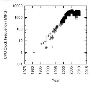
Figure 5.14: MIPS/Clock-Frequency Trend for Intel CPUs
