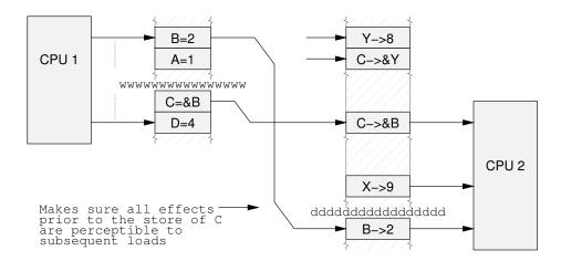
Figure 13.9: Data Dependency Barrier Supplied
