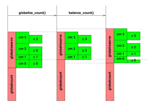
Figure 4.14: Schematic of Globalization and Balancing
