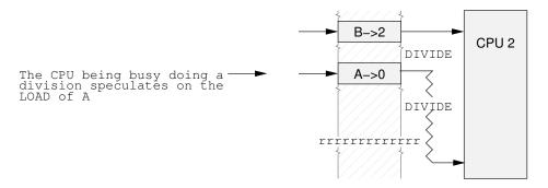
Figure 13.15: Speculative Load and Barrier
