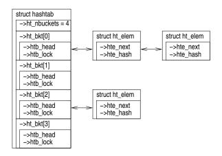
Figure 9.2: Hash-Table Data-Structure Diagram
