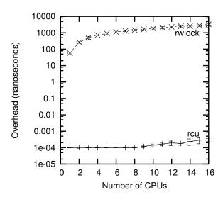
Figure 8.23: Performance Advantage of RCU Over Reader-Writer Locking
