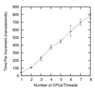
Figure 4.3: Atomic Increment Scalability on Nehalem
