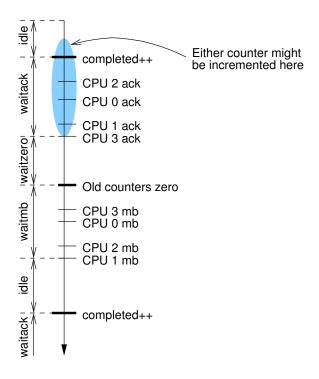
Figure D.64: Preemptible RCU State Machine Timeline
