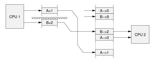
Figure 13.10: Read Barrier Needed
