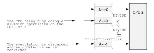
Figure 13.16: Speculative Load Cancelled by Barrier
