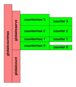
Figure 4.11: Simple Limit Counter Variable Relationships
