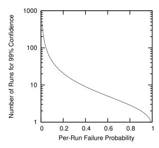
Figure 10.4: Number of Tests Required for 99 Percent Confidence Given Failure Rate
