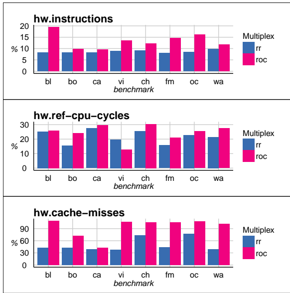
Figure 4: Accuracy in multiplexing strategies (round-robin, rate-of-change) with respect to baseline trace for select hardware events (more is better).
