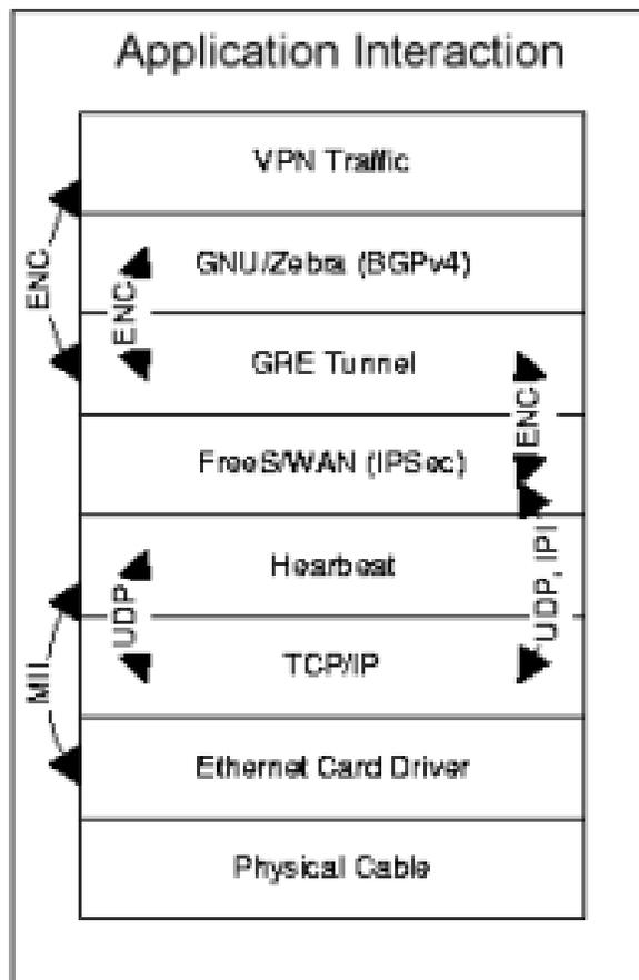
We have two Secure Gateways, each with a connection to the internet. Ideally, each would have its own link to the Internet, preferably redundant, but you could share the link if needed. Each gateway also has a connection to the local lan, which Heartbeat sends keep-alives over. If possible, use a Null-modem cable between each pair of gateways for out of band keep alives. If this isn't possible, Heartbeat also supports UDP keep-alives over any network interface.
