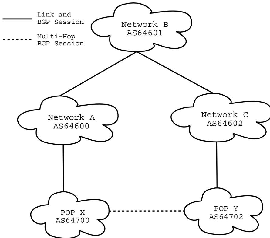
Figure 2: Network Diagram – Points of Presence
