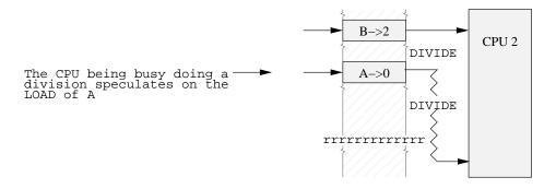
Figure 12.15: Speculative Load and Barrier
