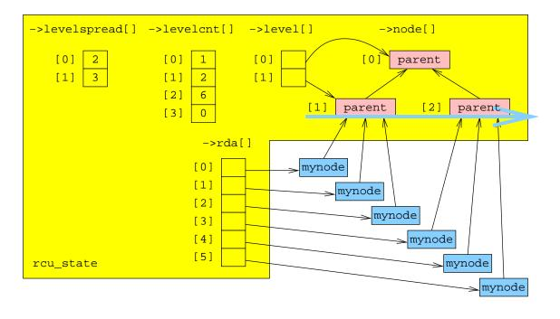
Figure D.52: Scanning Leaf rcu\_node Structures
