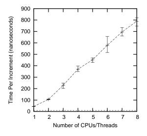
Figure 4.3: Atomic Increment Scalability on Nehalem
