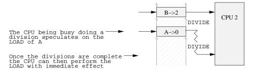
Figure 12.14: Speculative Load
