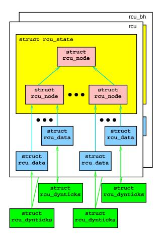
Figure D.17: Hierarchical RCU State With Dynticks
