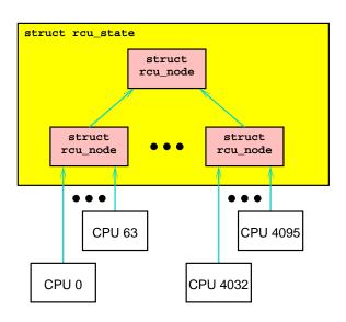
Figure D.15: Hierarchical RCU State 4,096 CPUs
