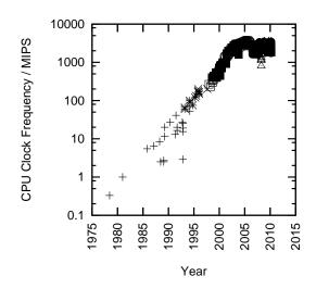
Figure 1.1: MIPS/Clock-Frequency Trend for Intel CPUs
