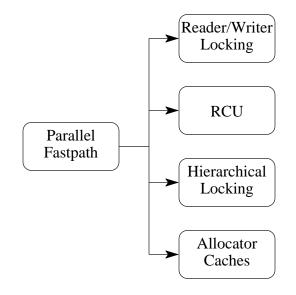
Figure 5.23: Parallel-Fastpath Design Patterns
