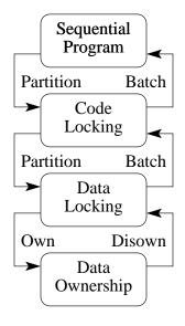
Figure 5.12: Design Patterns and Lock Granularity
