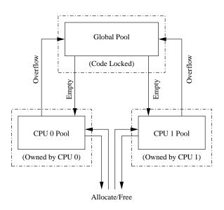
Figure 5.27: Allocator Cache Schematic
