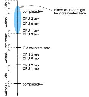
Figure D.64: Preemptable RCU State Machine Timeline
