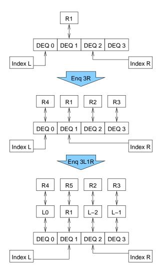
Figure 5.7: Hashed Double-Ended Queue After Insertions
