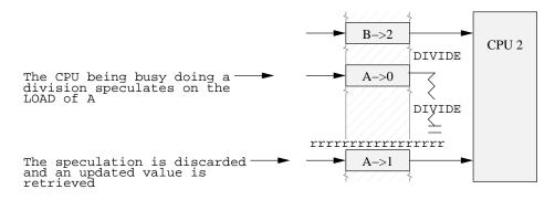
Figure 12.16: Speculative Load Cancelled by Barrier
