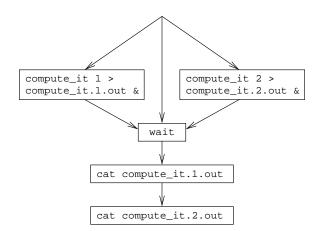
Figure 3.1: Execution Diagram for Parallel Shell Execution
