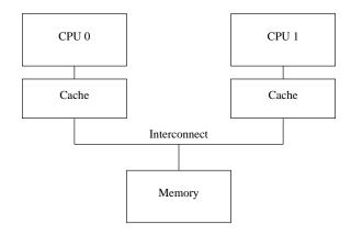
Figure 12.1: Modern Computer System Cache Structure
