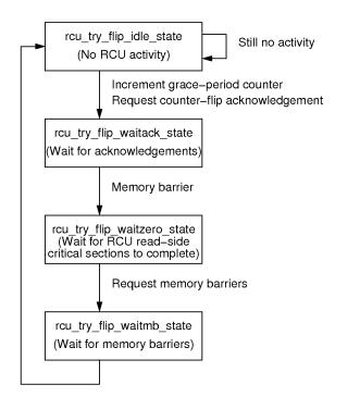
Figure D.63: Preemptable RCU State Machine
