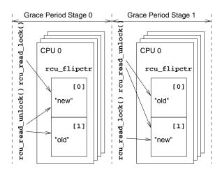
Figure D.61: Preemptable RCU Counter Flip Operation
