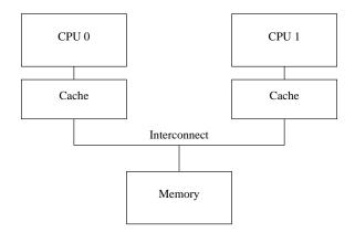
Figure C.1: Modern Computer System Cache Structure
