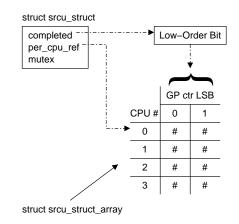
Figure D.5: SRCU Data-Structure Diagram
