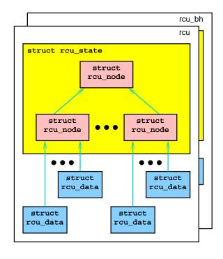
Figure D.16: Hierarchical RCU State With BH
