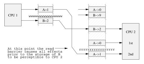
Figure 12.12: Read Barrier Supplied, Double Load
