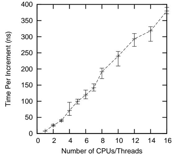
Figure 1: Atomic-Increment Overhead as Function of CPUs/Threads
